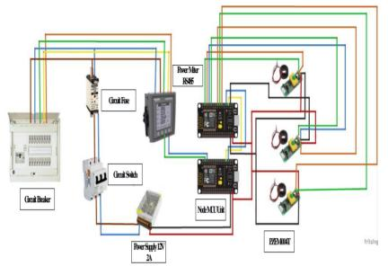
Figure 1: Schematic of IoT Smart Meter Control Box Hardware and Connection
