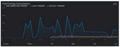
Figure 4: Example of a hotel room (35 sq.m.) energy consumption profile (W) of air conditioner, lighting, and an outlet for two days period
